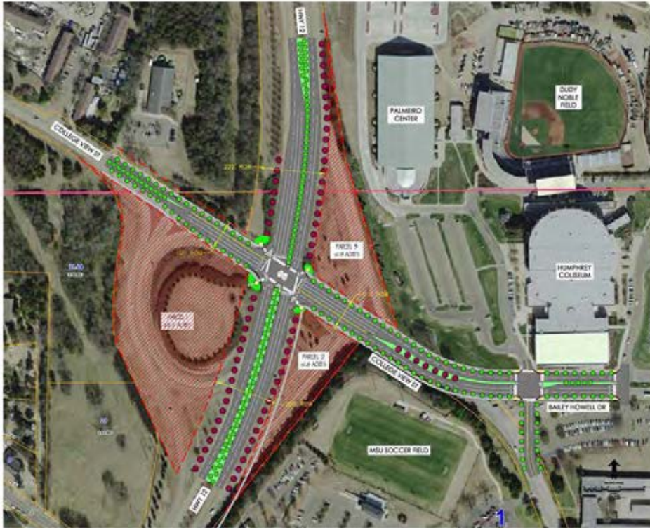
HWY 12 - COLLEGE VIEW STREET - PROPOSED IMPROVEMENTS PROPOSED AT-GRADE INTERSECTION & VACATED RIGHT-OF-WAY EXHIBIT
